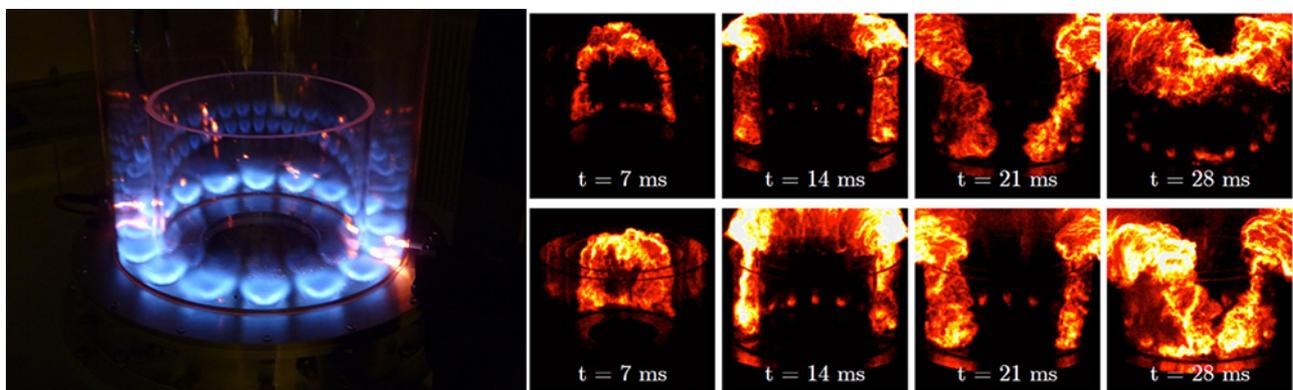
Figure 1: MICCA laboratory scale annular combustor (CNRS/EM2C) [1-6]
