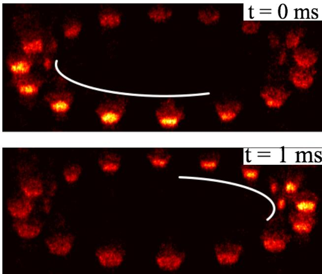
Figure 1: Azimuthal thermo-acoustics instabilities in the MICCA annular combustor [1-5]
