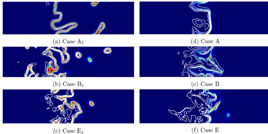
Fig. 1: instantaneous heat release rate fields on longitudinal cuts and contours of the progress variable (See (Suillaud et al. 2022) for details on legends and colorbar).
