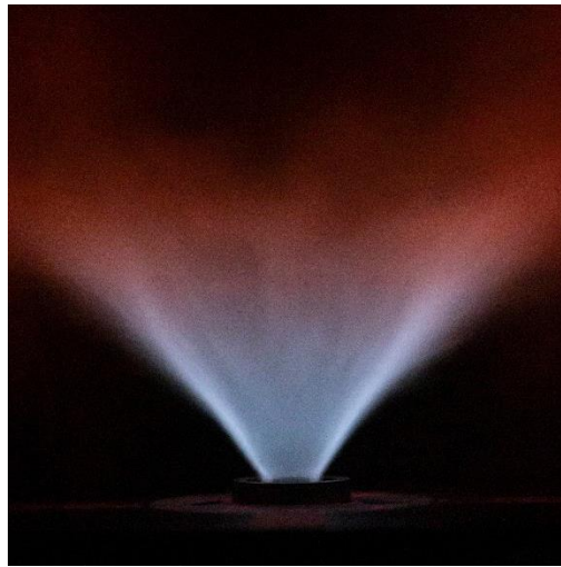
Photography of a stabilized hydrogen-air flame above a double swirled co-axial injector from EM2C-CNRS.
